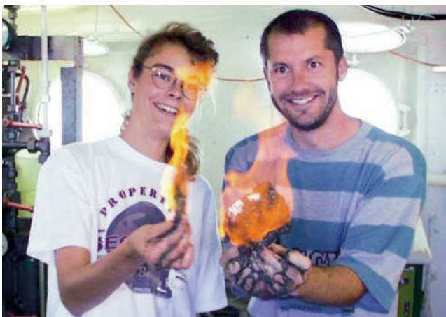
(b) Gas hydrates decompose when exposed to surface conditions and release natural gas, which can be ignited.
