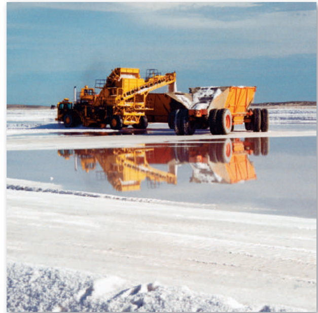
Figure 4.28 Mining sea salt. A salt mining operation at Scammon's Lagoon, Baja California, Mexico. Low-lying areas near the lagoon are allowed to flood with seawater, which evaporates in the arid climate and leaves deposits of salt that are then collected.
